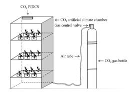
Fig. 1: CO<sub>2</sub> artificial climate chamber
